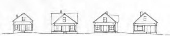
The relationships between the façade elements on each house are appropriately similar.
